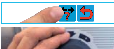
Press the selection button and scroll down using the central dial
