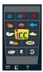
You can access the iCookingControl mode by selecting your required results, for example by selecting poultry, side dishes or fish.
