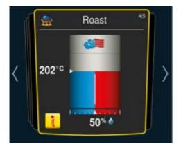
The i button appears as soon as a decision was made or a setting is being adjusted in the background. Press the i button or press the central dial to open the iCC Monitor in the iCC cockpit.
