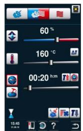
You enter the Combisteamer mode by pressing the button "steam", "combination" or "convection". See the Combi-steamer mode section for a description.
