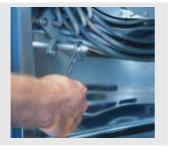
Loosen the union nut on the moistening nozzle (turn anti-clockwise – spanner size 15).
