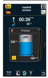
You can open the iCC cockpit by pressing the iCC cockpit button or it will open automatically after 10 seconds.
