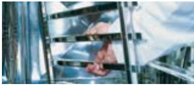
Insert hanging rack and fix hose with wire hooks
