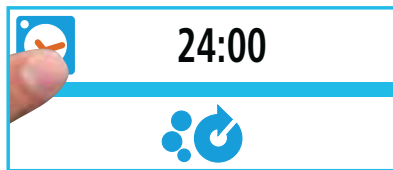
Press the clock button and enter the operating hours using the central dial
