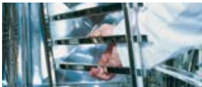
Remove descaler accessories, insert air baffle and left hanging rack, and lock in place
